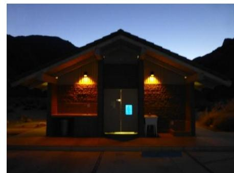
After installation of lower-wattage lamps in fully-shielded fixtures, the lights on the restroom building now provide plenty of light for campers to find their way, without light trespass into nearby campsites, or the glare that disturbed night-sky viewing, not to mention wildlife.
