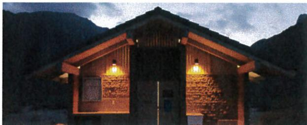
*Shielded light fixtures direct light downward, where it's needed.*
