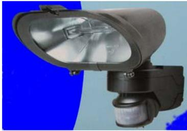
This light is sold as being “dark sky friendly”. It has a reflector that is shaped to direct the light downwards, and has a sensor which switches it on when someone is nearby. It should be fitted with a lamp of 150W or less. It also provides reduced illumination dusk to dawn for courtesy and full power on presence detection.
